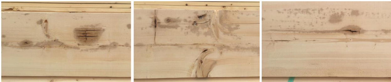
FIGURE 5 – AN EXAMPLE OF “DIESEL ROT” IN A NEWLY CUT SPRUCE BOARDS, “DIESEL ROT” IS A CURRENTLY UNIDENTIFIED STAIN ENCOUNTERED DURING THE MILLING OF BOTH HEALTHY AND SPRUCE BEETLE-KILLED TREES. PHOTO CREDIT: CANADIAN FOREST PRODUCTS LTD.
